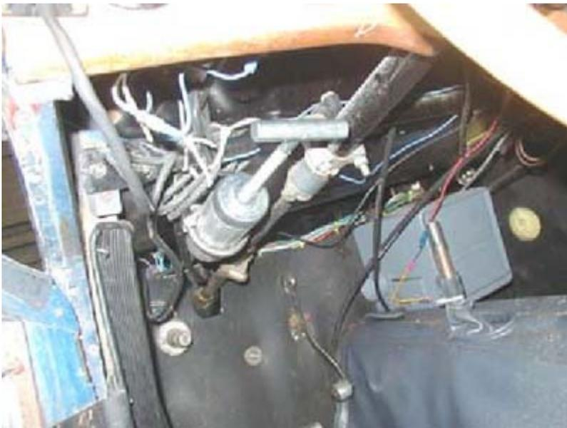
Alemite Greaser mounted in drivers side of +4 under dash.
