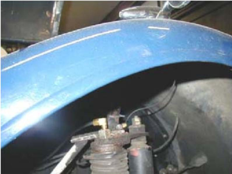
Of course the King Pins must be drilled so that the grease comes out in the stub axle. This set up is one to accomplish when you determine new King Pins and Bushings are to be installed.
