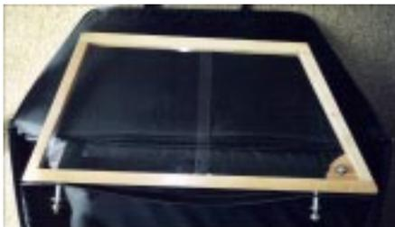
location of mounting studs and length of the two pieces of glass. I ripped and planed the ash to size. The bottom pieces are 15/16 x 15/16, sides and tops are 3/4 x 15/16 in cross section. I laid the pieces on the drawing to mark length
