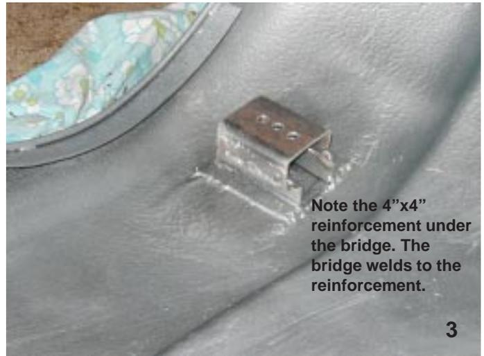
**Step 5:** Remove the fender support brace (the curved piece of flat steel that supports the fender), cut about two inches out of its height, and reweld it together so that when put back on the car it sits just under the new bridge structure. Adjust the length of the fender support so that the top of the fender is level when viewed from the front. If you cut off a little too much, add a few washers to adjust the top of the fender so that it is correct.
