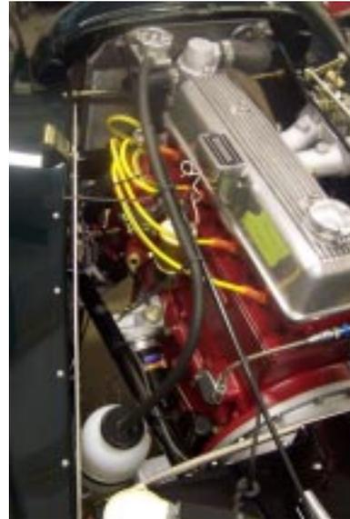
**Step 3 - the overflow hose:** Run a hose from the nipple on the filler neck down the radiator stay rod and into the bottle. Make sure the hose goes all the way to the bottom of the bottle.
