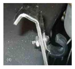
less nut and bolt (picture 4). The rod should then rest inside this clamp and with a little bending of the clamp it can be held firmly but easily removed. In some models of Morgans and on some sides you may have to bend the rod slightly to get it round the carbs but this is easily done across the knee.
