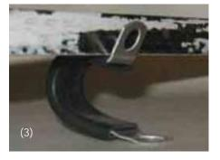
a hacksaw (picture 3). Then drill a hole through the hood latch nearest the front and attach the cut conduit clamp to the inside of the bonnet latch with a stain-
